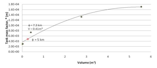
**Figure 6.** Sampling of Scorpius<sup>®</sup> [USA] Composite Tanks (1.7 MPa MEOP (250 psi)): Volume vs. Tank mass factor. Reprinted with permission from ref. [39]. Copyright 2010 American Institute of Aeronautics and Astronautics.
