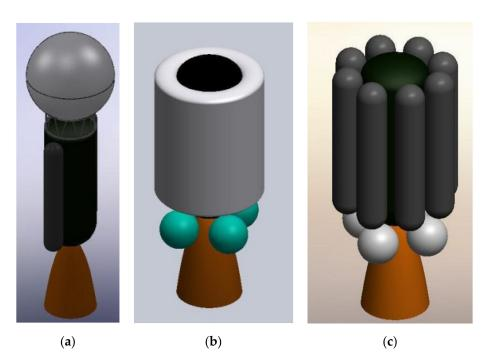
**Figure 5.** Examples of hybrid upper stage arrangements: (a) Serial; (b) Toroidal; (c) Multiple tanks. Reprinted with permission from ref. [9]. Copyright 2011 American Institute of Aeronautics and Astronautics.
