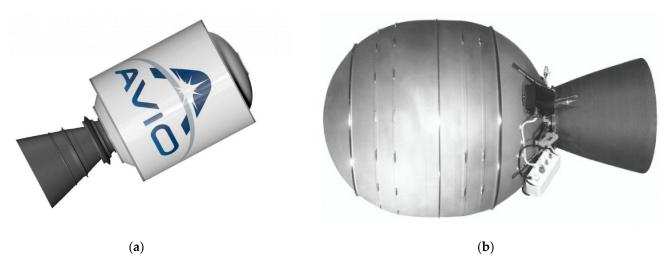
**Figure 4.** Examples of solid rocket upper stages: (**a**) Avio Zefiro 9 (Vega); (**b**) Northrop Grumman Star 48 (Minotaur IV). Note the very compact length to diameter ratio. (**a**) Reprinted with permission from https://www.avio.com/ (accessed on 9 July 2021). Copyright 2021 Avio. (**b**) Reprinted with permission from ref. [34]. Copyright 2016 Northrop Grumman.
