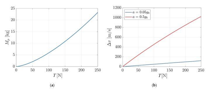
**Figure 1.** Examples of hybrid rocket design limits for satellites: (a) Propellant mass vs. thrust; (b) Velocity increment vs. thrust for different maximum allowable accelerations. Reprinted with permission from ref. [30]. Copyright 2020 American Institute of Aeronautics and Astronautics.
