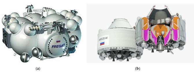
**Figure 2.** Examples of liquid propelled space tugs: (**a**) NPO Lavochkin Fregat (Soyuz/Zenit); (**b**) GKNPTs Khrunichev Briz-M (Proton). Note the extremely compact length to diameter ratio and the propellant tank arrangement. Copyright: publicly available pictures on the internet.
