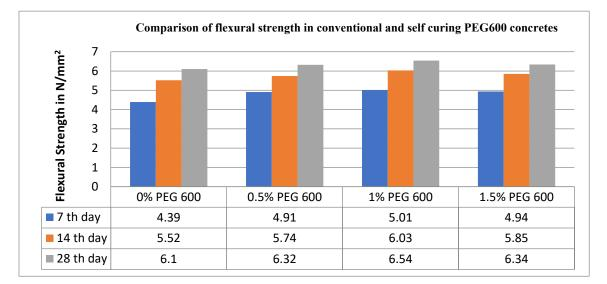
Figure 5. Comparison of flexural strengths of Conventional and PEG-600 concretes.
