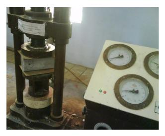
Figure 3. Split tensile test setup.
