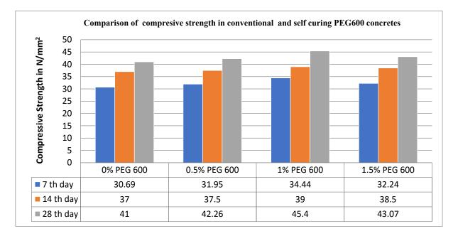
Figure 4. Comparison of compressive strength in conventional and PEG-600 concretes.
