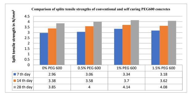
Figure 6. Comparison of split tensile strengths of Conventional and PEG-600 concretes.
