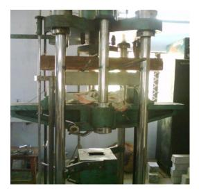
Figure 2. Flexural strength testing setup.
