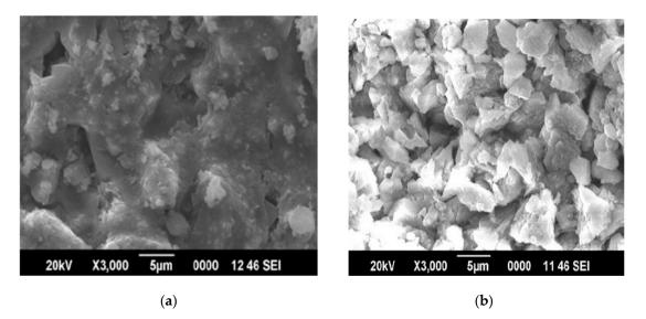
Figure 7. (a) Conventional concrete, (b) self-curing concrete.
