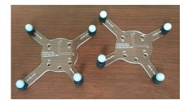
Figure 10. Fabricated calibration rigid bodies for the UR5 (left) and UR10 (right) manipulators.
