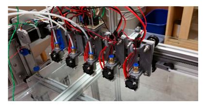
**Figure 2.** X-axis gantry assembly.  $5 \times$  Hexagon Full-Metal 12 V hot ends are shown fixtured to their respective 'Z-Height Bed Leveling Adjustment' part files. As shown, dovetail leveling mechanisms are attached to the machined aluminum plate (3.175 mm  $\times$  25.4 mm  $\times$  295.75 mm) with Hexagon nozzle diameter cylindrical axis spaced 55 mm.
