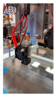
**Figure 3. (A)** Top printer gantry with fixtured 5 NEMA 17 extruder drive motors and respective "MOST Bowden Extruder Drive" printed components; **(B)** hexagon hot-end assembly detail with "Z-Height Bed Leveling Adjustment" dovetails.
