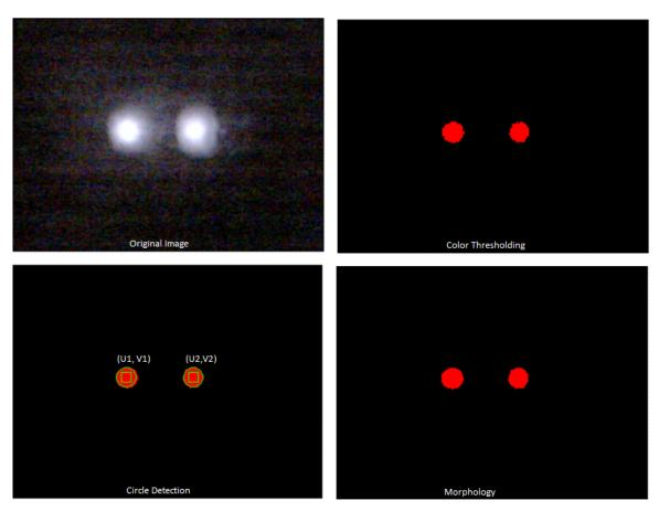
Figure 2. Blob detection and tracking algorithm outputs.
