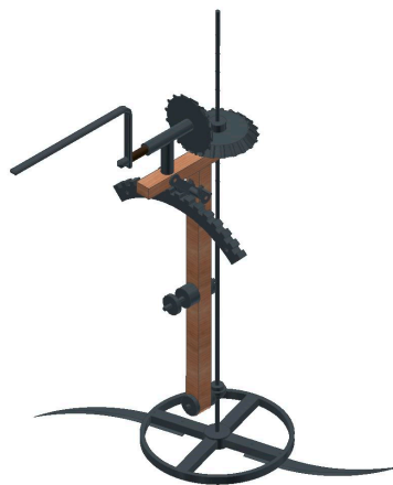
Figure 9. Axonometric view of the two-blade cutting mechanism.
