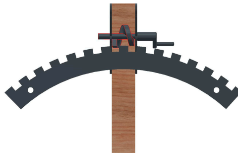
Figure 8. Details of the gear between the worm screw and the quarter gear.
