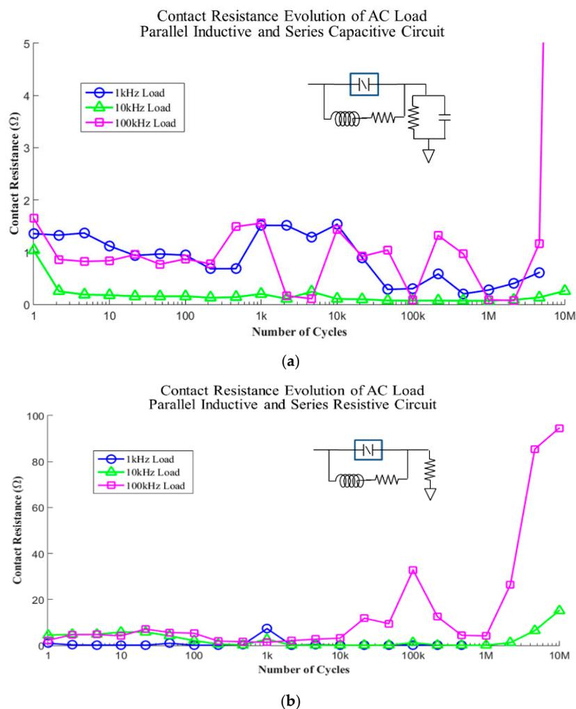
**Figure 5.** Contact resistance versus number of cycles measurements at three AC frequencies (1, 10 and 100 kHz) for (a) an external load of parallel resistive-inductive RL and series resistive-capacitive RC; and (b) parallel RL and series resistive (R) added to micro-contacts.
