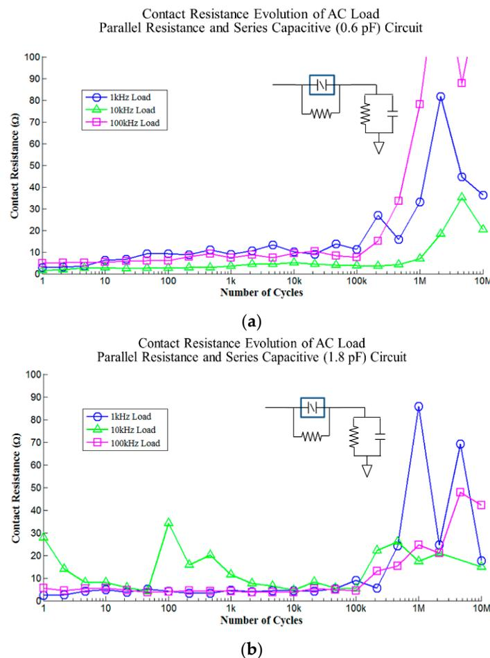
**Figure 6.** Contact resistance versus number of cycles measured at three AC frequencies (1, 10 and 100 kHz) for (a) an external load of parallel R and series RC; and (b) parallel R and series RC (larger C this time) added to micro-contacts.
