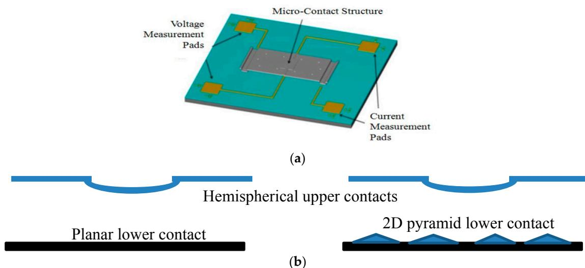
**Figure 2.** (a) Schematic of a micro-contact fabricated with a hemispherical contact bump on the lower side of the upper support beam; (b) Physical representation of different lower pads used in this study.
