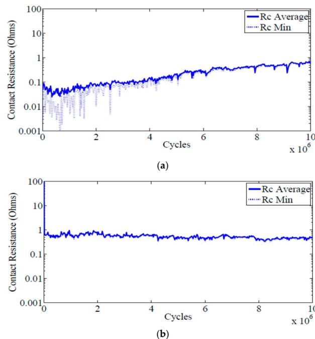
**Figure 7.** Contact resistance versus number of cycles measured for (a) planar; and (b) 2D pyramid. For all plots, the contact resistance ( $R_C$ ) average is the average of the last five data points at  $\sim 200 \mu\text{N}$  of contact force, and  $R_C$  min is the minimum contact resistance measured.
