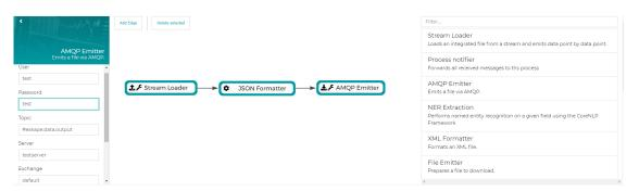
**Figure 11.** Data extraction using an Advanced Message Queuing Protocol (AMQP) emitter in a processing pipeline.
