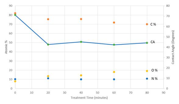
**Figure 2.** Quantitative XPS (at %) and water contact angle (CA) results for polybenzimidazole (PBI) (Celazole<sup>®</sup>) treated with UV photo-oxidation as a function of treatment time.
