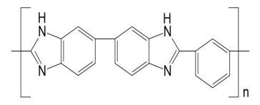
Figure 1. Molecular structure of polybenzimidazole (PBI).
