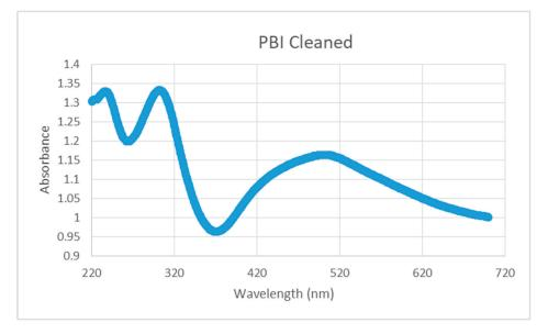
Figure 7. UV-visible photoabsorption spectrum of polybenzimidazole (PBI) (Celazole®).
