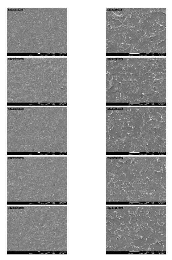
**Figure 6.** SEM surface topographic images at  $500 \times$  and  $2000 \times$  magnification after 0, 20, 40, 60, and 80 min treatment with UV photo-oxidation.
