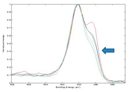
**Figure 4.** Overlapped N 1s spectra for cleaned control and UV photo-oxidized PBI samples. The arrow indicates increasing treatment time for 0, 20, 40, 60, and 80 min.
