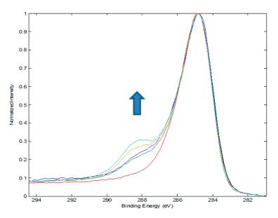
**Figure 3.** Overlapped C 1s spectra for cleaned control and UV photo-oxidized PBI samples. The arrow indicates increasing treatment time for 0, 20, 40, 60, and 80 min.
