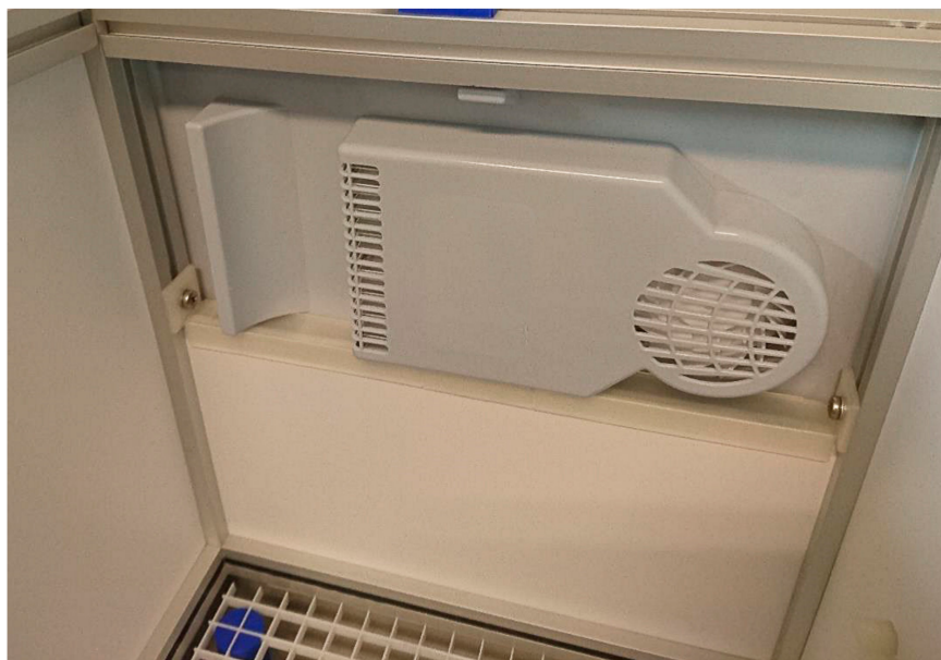
Figure 7. Peltier module-based cooling system installed in the chamber.
