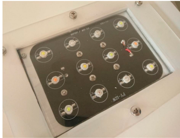
Figure 9. Lighting unit bottom side – LEDs soldered onto a PCB (printed circuit board) plate.
