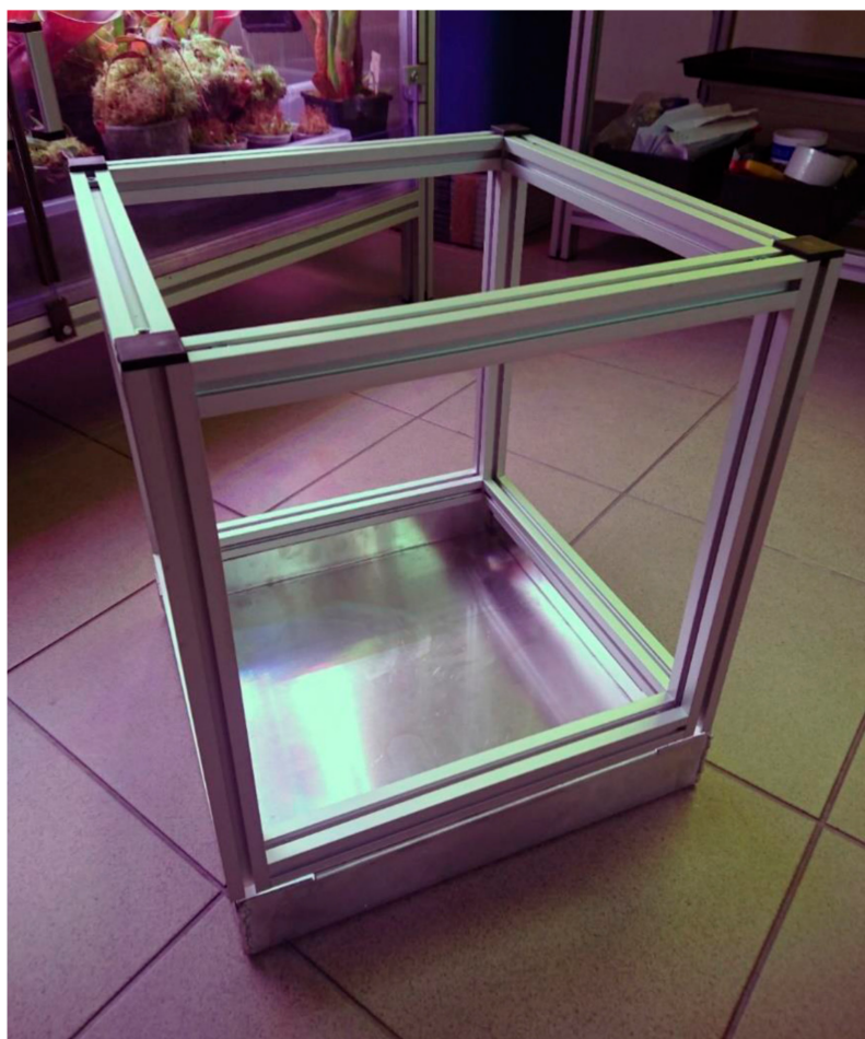
Figure 4. Aluminum profile frame of the chamber.
