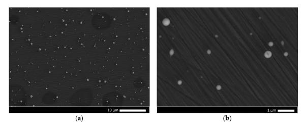
**Figure 7.** SEM photomicrographs of nanoparticles electrosprayed from the hyaluronic acid solutions with concentration 2.5 mg/mL under 30 kV: (**a**) magnification 4000×; (**b**) magnification 25,000×.
