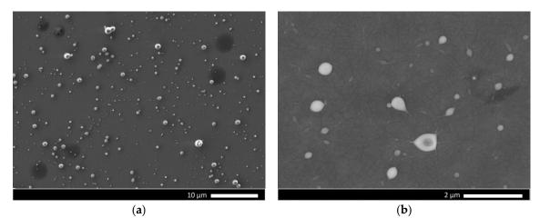
**Figure 11.** SEM photomicrographs of nanoparticles electrosprayed from the hyaluronic acid solutions with concentration 12.5 mg/mL under 30 kV: (**a**) magnification 4000×; (**b**) magnification 25,000×.
