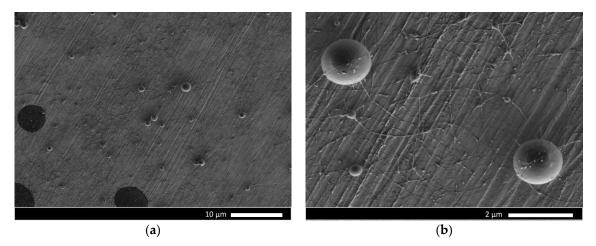
**Figure 12.** SEM photomicrographs of nanoparticles electrosprayed from the hyaluronic acid solutions with concentration 15.0 mg/mL under 30 kV: (**a**) magnification 4000×; (**b**) magnification 25,000×.
