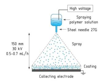
Figure 2. Principal scheme of the electrospraying process and technological parameters.
