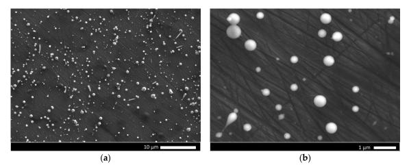
**Figure 8.** SEM photomicrographs of nanoparticles electrosprayed from the hyaluronic acid solutions with concentration 5.0 mg/mL under 30 kV: (**a**) magnification 4000×; (**b**) magnification 25,000×.
