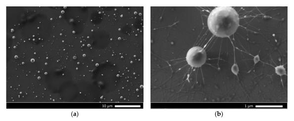
**Figure 10.** SEM photomicrographs of nanoparticles electrosprayed from the hyaluronic acid solutions with concentration 10.0 mg/mL under 30 kV: (**a**) magnification 4000×; (**b**) magnification 42,000×.
