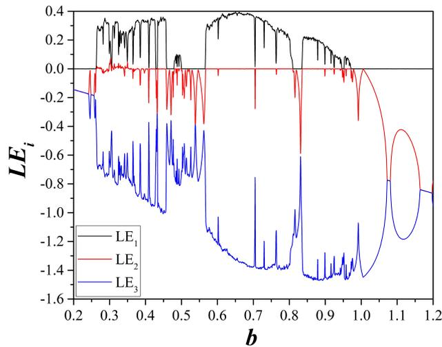
Figure 4. Spectrum of Lyapunov exponents of system (2), when varying  $b$ , for  $a = 4 \times 10^{-4}$ ,  $c = 3.846 \times 10^{-4}$  and  $d = e = 1$ .
