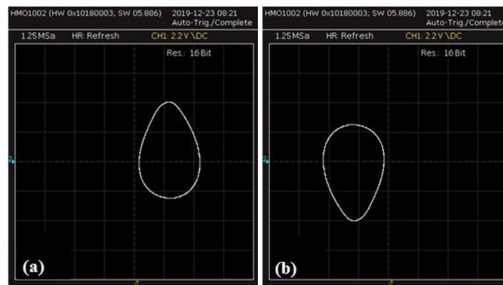
**Figure 6.** (a,b) Experimentally observed coexisting period-1 phase portraits of  $v_{C_1}$  versus  $v_{C_2}$ , for  $a = 4 \times 10^{-4}$ ,  $c = 3.846 \times 10^{-4}$ ,  $d = e = 1$  and  $b = 0.2$  ( $R_b = 50 \text{ k}\Omega$ ).
