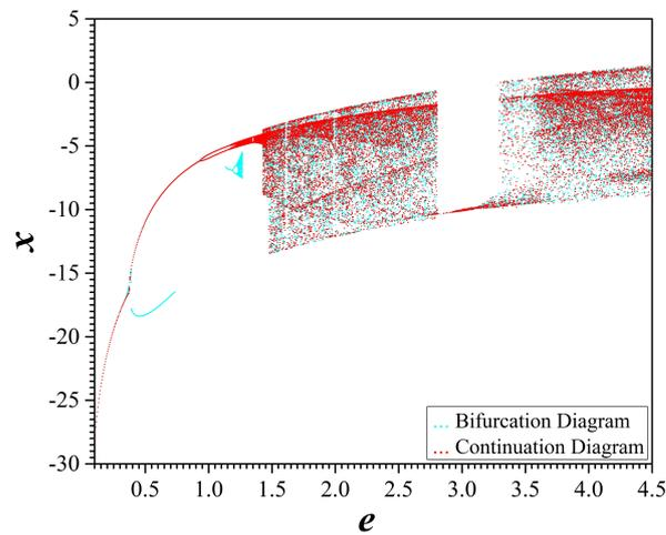
**Figure 14.** Bifurcation diagram (cyan) and continuation diagram (red) of system (2), when parameter  $e$  is increased, for  $a = 4 \times 10^{-4}$ ,  $b = 1$ ,  $c = 3.846 \times 10^{-4}$  and  $d = 1$ , when parameter  $e$  is increased.
