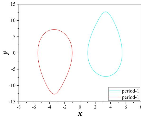
**Figure 13.** Coexisting attractors of system (2), for  $a = 4 \times 10^{-4}$ ,  $b = 1$ ,  $c = 3.846 \times 10^{-4}$ ,  $e = 1$  and  $d = 19$ . With cyan color and for  $(x_0, y_0, z_0) = (0, 0.1, 0)$  a period-1 attractor, while with red color and  $(x_0, y_0, z_0) = (-5.5160634, 0, 1.737452)$  a symmetric period-1 attractor.
