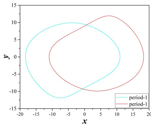
**Figure 15.** Coexisting attractors of system (2), for  $a = 4 \times 10^{-4}$ ,  $b = 1$ ,  $c = 3.846 \times 10^{-4}$ ,  $d = 1$  and  $e = 0.50$ . With cyan color and for  $(x_0, y_0, z_0) = (0, 0.1, 0)$  a period-1 attractor, while with red color and  $(x_0, y_0, z_0) = (-10.969297, 0, 4.5870237)$  a symmetric period-1 attractor.
