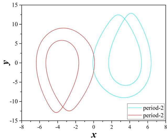
**Figure 12.** Coexisting attractors of system (2), for  $a = 4 \times 10^{-4}$ ,  $b = 1$ ,  $c = 3.846 \times 10^{-4}$ ,  $e = 1$  and  $d = 15$ . With cyan color and for  $(x_0, y_0, z_0) = (0, 0.1, 0)$  a period-2 attractor, while with red color and  $(x_0, y_0, z_0) = (-5.3107692, 0, 1.7241613)$  a symmetric period-2 attractor.
