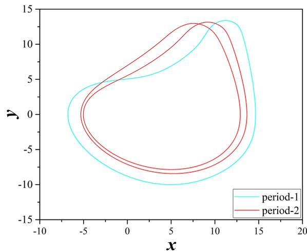
**Figure 16.** Coexisting attractors of system (2), for  $a = 4 \times 10^{-4}$ ,  $b = 1$ ,  $c = 3.846 \times 10^{-4}$ ,  $d = 1$  and  $e = 1.15$ . With cyan color and for  $(x_0, y_0, z_0) = (0, 0.1, 0)$  a period-1 attractor, while with red color and  $(x_0, y_0, z_0) = (-5.3168311, 0, 4.9638148)$  a period-2 attractor.
