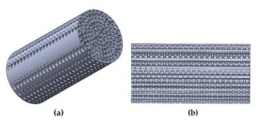
Figure 8. Drawing (a) and cross-section (b) of the catalyst made in the SolidWorks software.
