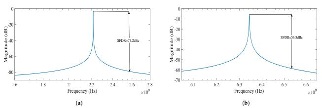
Figure 11. Spectrum of the (a) DAC-based DCO at 2.2 GHz, (b) Controller-based DCO at 6.4 GHz.
