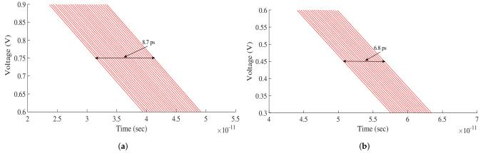
Figure 10. Jitter of the (a) DAC-based DCO at 2.2 GHz, (b) Controller-based DCO at 6.4 GHz.
