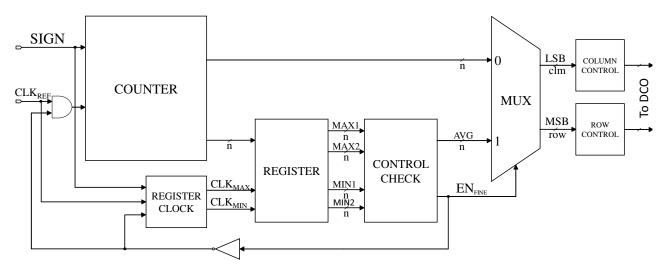
Figure 7. Block diagram of the controller.
