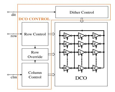
Figure 5. Block diagram of controller-based DCO.
