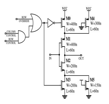
Figure 6. Schematic of the delay cell.
