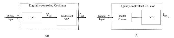
Figure 1. DCO controlled by (a) DAC, and by a (b) digital controller.
