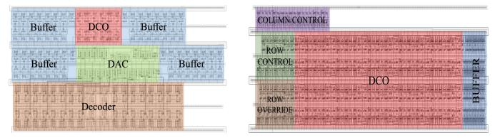
(a) (b) Figure 8. Layout of the (a) DAC-based DCO, (b) Controller-based DCO.
