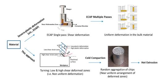
**Figure 1.** Comparison between ECAP as an existing SPD technique and the newly-explored TID processing method as a new SPD technique [18].
