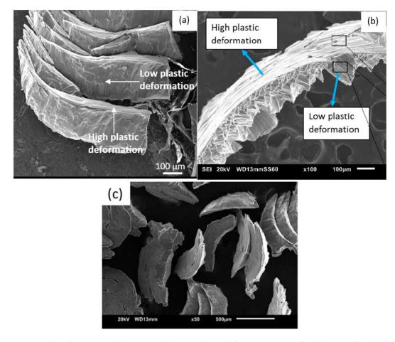
**Figure 2.** Micrographs of Mg-material turnings, showing plastic deformation zones for (**a**) AZ91 alloy, (**b**) Mg/Fe<sub>3</sub>O<sub>4</sub> nanocomposites, and (**c**) ZK60 alloy. [18,24,25].
