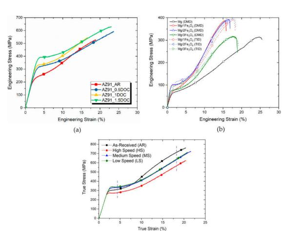
**Figure 4.** Compressive stress–strain charts associated with TID Mg materials and their improvement over conventionally-processed materials for (**a**) AZ91 alloy, (**b**) Mg/Fe<sub>3</sub>O<sub>4</sub> nanocomposites, and (**c**) ZK60 alloy [18,24,25].
