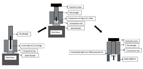
Loose turnings before compaction
