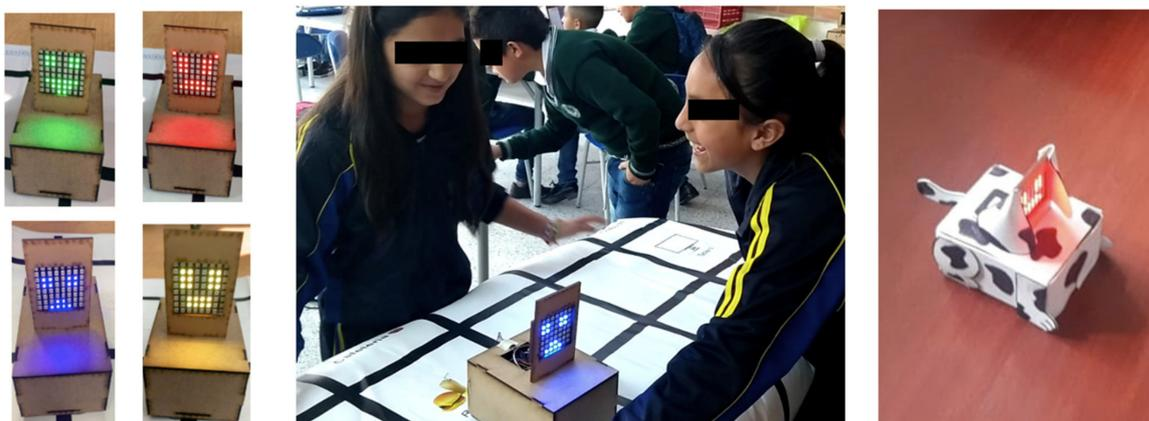
**Figure 3.** Actor robots used in the second experiment. These robots had a screen to enhance the emotional expressiveness of the robots. They also had a speaker for audio playback.
