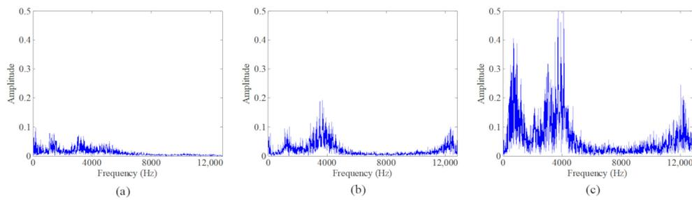
**Figure 4.** Spectrum images of bearing 4 in three operation stages: (a) Status 1, (b) Status 2, and (c) Status 3.
