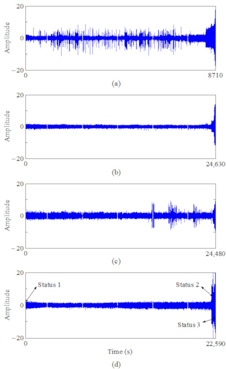
Figure 3. Vibration signals of four bearings: (a) bearing 1, (b) bearing 2, (c) bearing 3, and (d) bearing 4.
