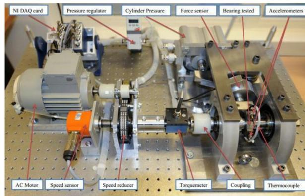
Figure 2. Overview of the experimental setup.
