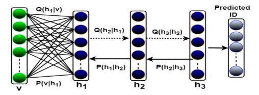
Figure 4. The main architecture of the developed DBN model for addressing person ReID problems.
