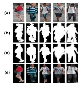
**Figure 6.** Some examples of applying the proposed person's body segmentation procedure: (**a**) original images, (**b**) body mask generated from the Mask R-CNN, (**c**) body mask generated from the enhanced Mask R-CNN using the GrabCut algorithm, and (**d**) the final detected person's body.
