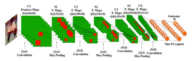
Figure 3. The architecture of the developed CNN model for addressing person ReID problems.
