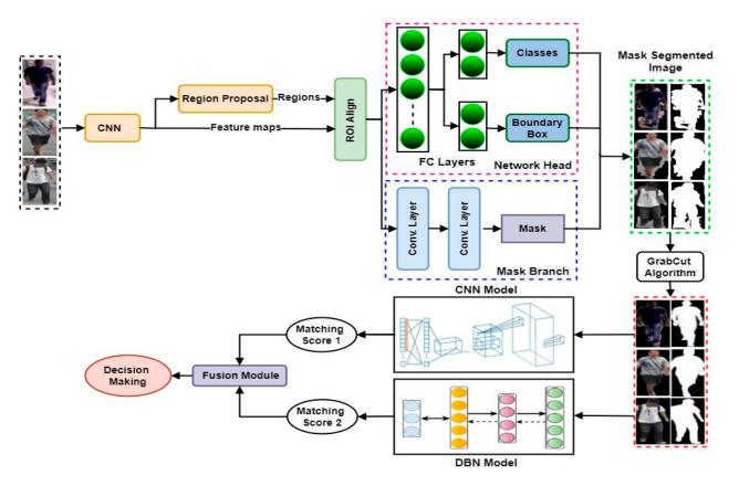
Figure 1. The overall structure of the proposed ReID-DeePNet system.
