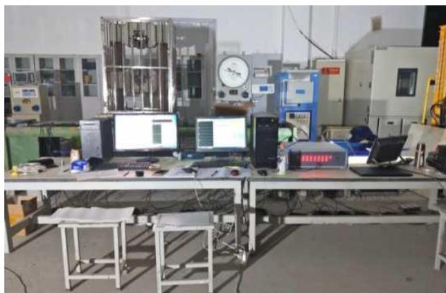
Figure 1. Tensile testbed of steel strand.
