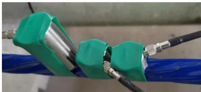
Figure 3. Acoustic emission sensors.
