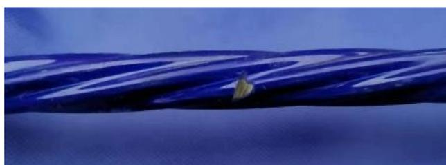
Figure 2. Prefabricate a notch on the steel strand.
