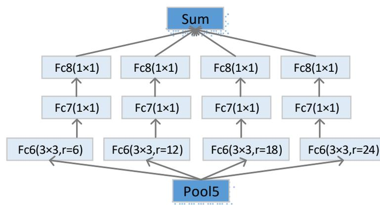
**Figure 3.** Illustration of ASPP with different atrous rates in each branch.
