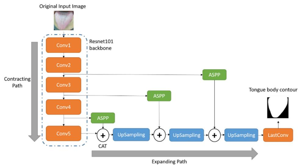
Figure 5. Overall architecture of semantic-based CNNs (SegTongue).
