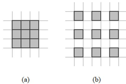
**Figure 2.** A schematic diagram of the atrous convolution at different expansion rates. (a)  $r = 1$ ; (b)  $r = 2$ .
