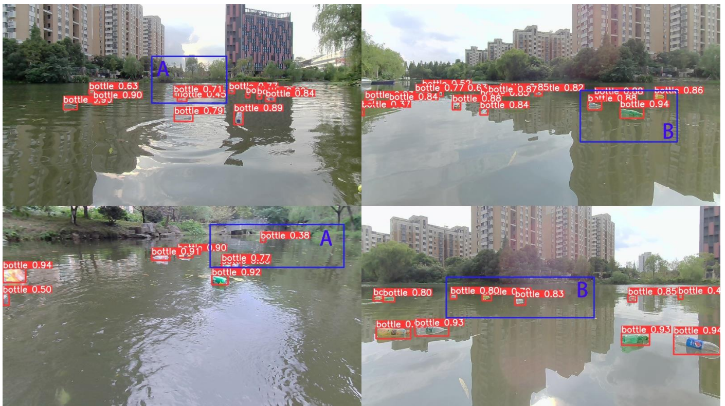
Figure 14. Sample images of the FloW-Img public dataset, revealing some shortcomings of YOLOv5_CBS (e.g., when multiple small objects are present in the images, or when the density of the target objects is high, this may result in a low detection rate and low confidence level, as shown in areas A, or when reflections on the water surface exist, then part of the prediction box may treat the reflection as an object too, or a bigger prediction box, including the reflection, may be formed, as shown in areas B).
