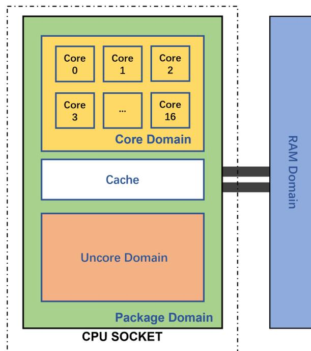
**Figure 9.** RAPL domain match part of our CPU socket. The energy consumption of the core measured by pyJoules is the sum of the CPU core energy consumption, the energy consumption of the packages is the wall CPU energy consumption, and the energy consumption of the uncore is the energy consumption of the integrated GPU.
