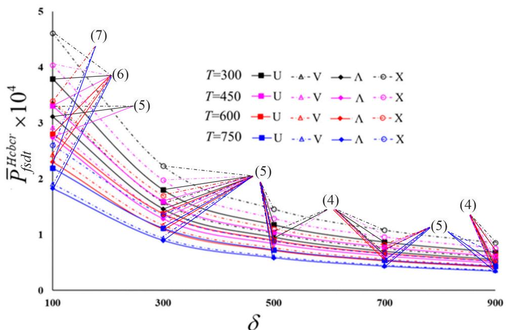
Figure 6. Distribution of  $\bar{P}_{fsdt}^{Hcbr}$  for nanocomposite cylindrical shells with various models versus the  $\delta$  for different temperatures.
