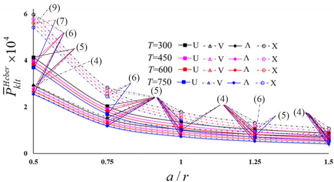
**Figure 7.** Distribution of  $\bar{P}_{klt}^{Hcbr}$  for nanocomposite cylindrical shells with various models in the thermal environment versus the  $a/r$ .
