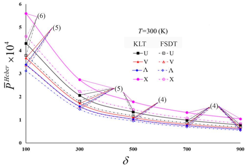
**Figure 3.** Distribution of  $\bar{P}_{fsdt}^{Hcbr}$  and  $\bar{P}_{klt}^{Hcbr}$  for nanocomposite cylindrical shells with various models versus the  $\delta$  at  $T = 300$  (K).
