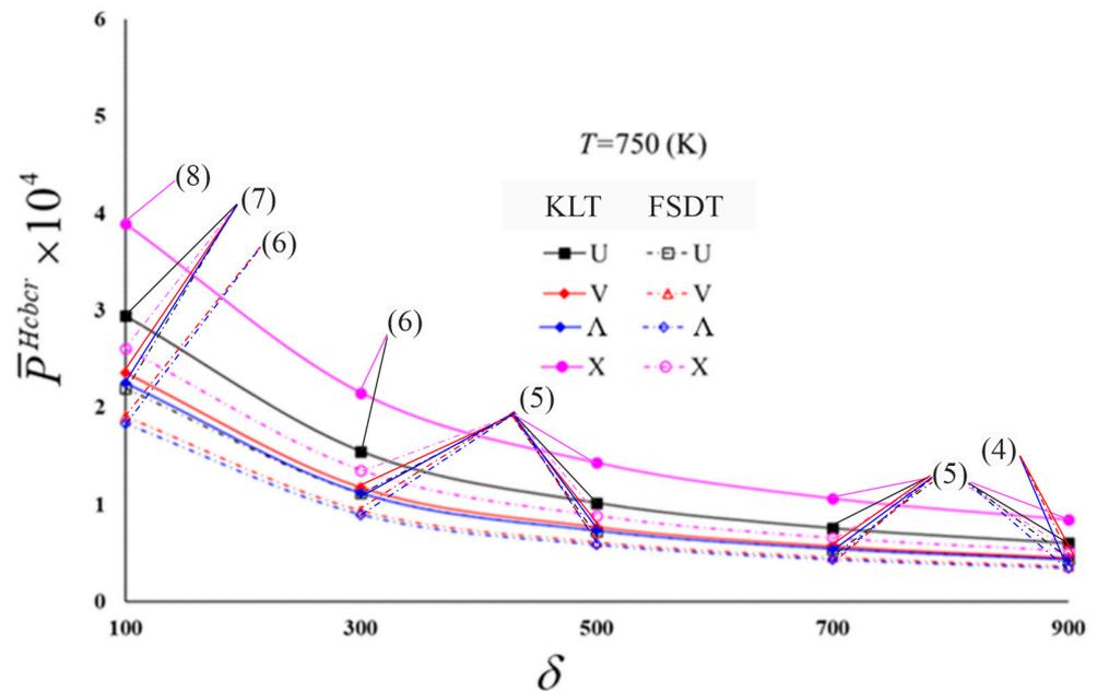
**Figure 4.** Distribution of  $\bar{P}_{fsdt}^{Hcbr}$  and  $\bar{P}_{klt}^{Hcbr}$  for nanocomposite cylindrical shells with various models versus the  $\delta$  at  $T = 750$  (K).
