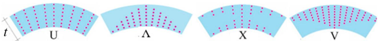
Figure 2. Shapes of the uniform and inhomogeneous distributions of CNTs in the thickness direction of the polymer matrix.
