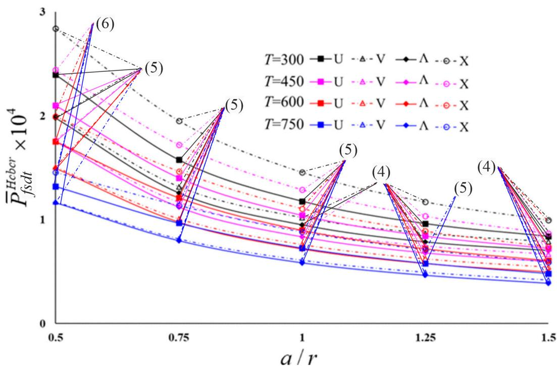
**Figure 8.** Distribution of  $\bar{P}_{fsdt}^{Hcbr}$  for nanocomposite cylindrical shells with various models in the thermal environment versus the  $a/r$ .
