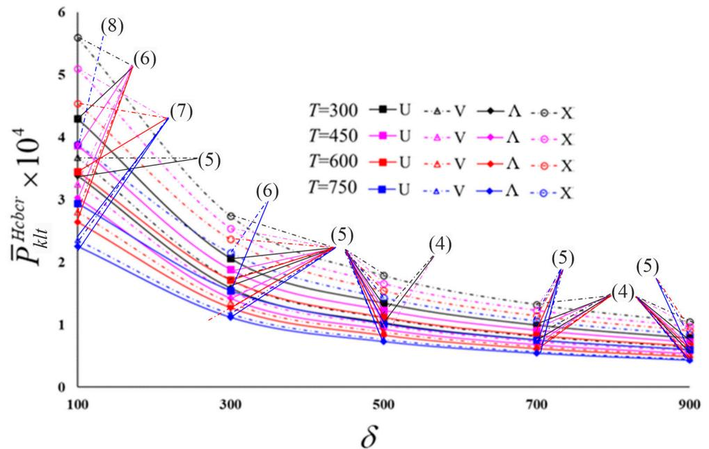
Figure 5. Distribution  $\bar{P}_{klt}^{Hcbr}$  for nanocomposite cylindrical shells with various models versus the  $\delta$  for different temperatures.
