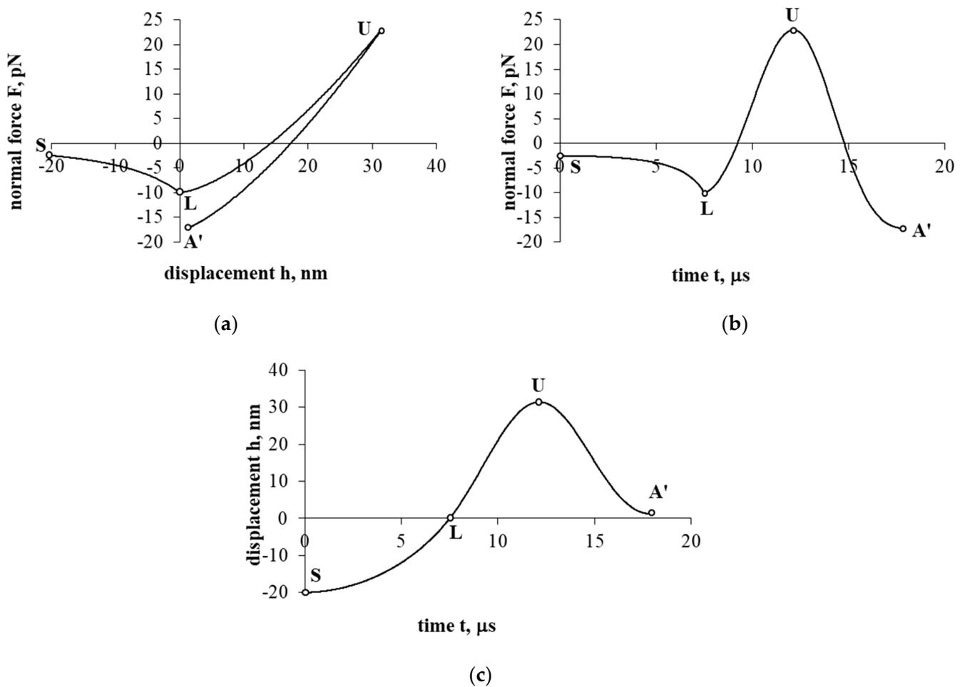
**Figure 2.** The first part of the investigation of the adhesive–elastic interaction. The electrostatic double layer force and the drag force are not considered. Dependence of force on displacement (a) and time (b); dependence of displacement on time (c).
