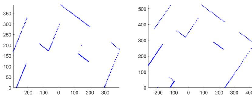
Figure 3. Visualization of laser range data for both real sensor RSD (left) and virtual sensor VSD (right).
