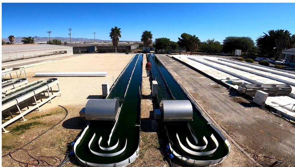
**Figure 1.** Raceway photobioreactors modeled in this work.
