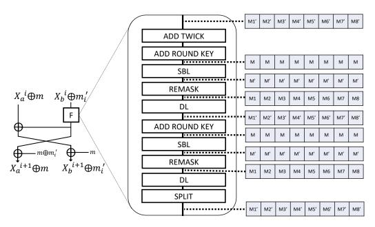
Figure 6. Proposed masking method.
