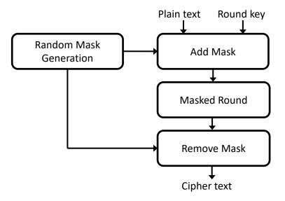
Figure 5. Masking step on FEA.
