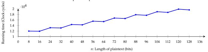
Figure 3. Differences of clock cycles depending on input *n* with AVR processor.
