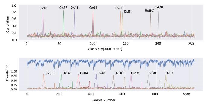
Figure 8. Top: correlation attack results, bottom: correlation test results.
