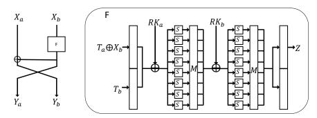
Figure 1. Feistel based round structure of FEA.
