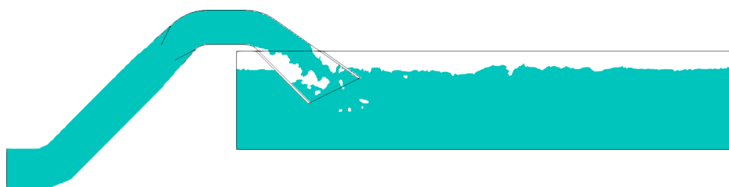
Figure 4. Bubbles inside the siphon when calculating from initial condition (28)–(30). Front part of a cut at z = 0 m.
