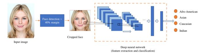
**Figure 3.** Outline of the proposed solution. The face region is extracted using an off the shelf face detector and it is further enlarged. A convolutional neural network is used to extract the relevant features and determine the race.
