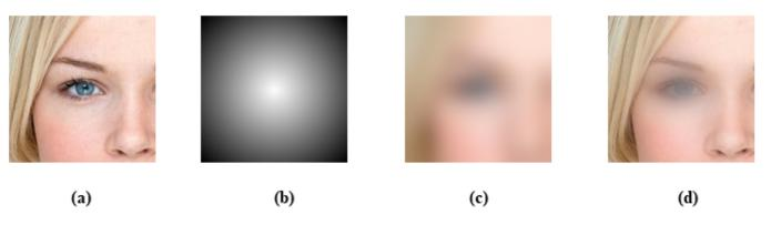
**Figure 6.** Radial blur: the input region of interest (**a**) is combined with the blurred region of interest (**c**), based on the weights defined by the blur mask (**b**). The result is illustrated in subfigure (**d**).
