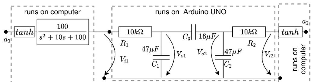
Figure 4. Conceptual description of the controlled system.
