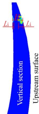
Figure 2. Parameters of local damage to the middle part of the dam.
