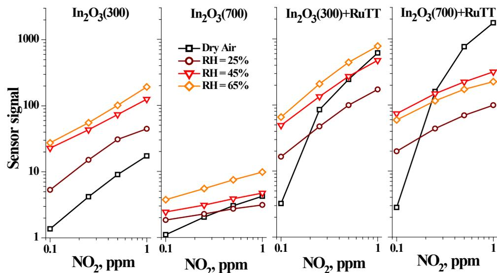
**Figure 10.** Dependence of the sensor signal of In<sub>2</sub>O<sub>3</sub>(300), In<sub>2</sub>O<sub>3</sub>(700) samples and hybrid materials based on them on the NO<sub>2</sub> concentration at different air humidity (relative humidity at 25 °C RH = 25, 45, 65%).
