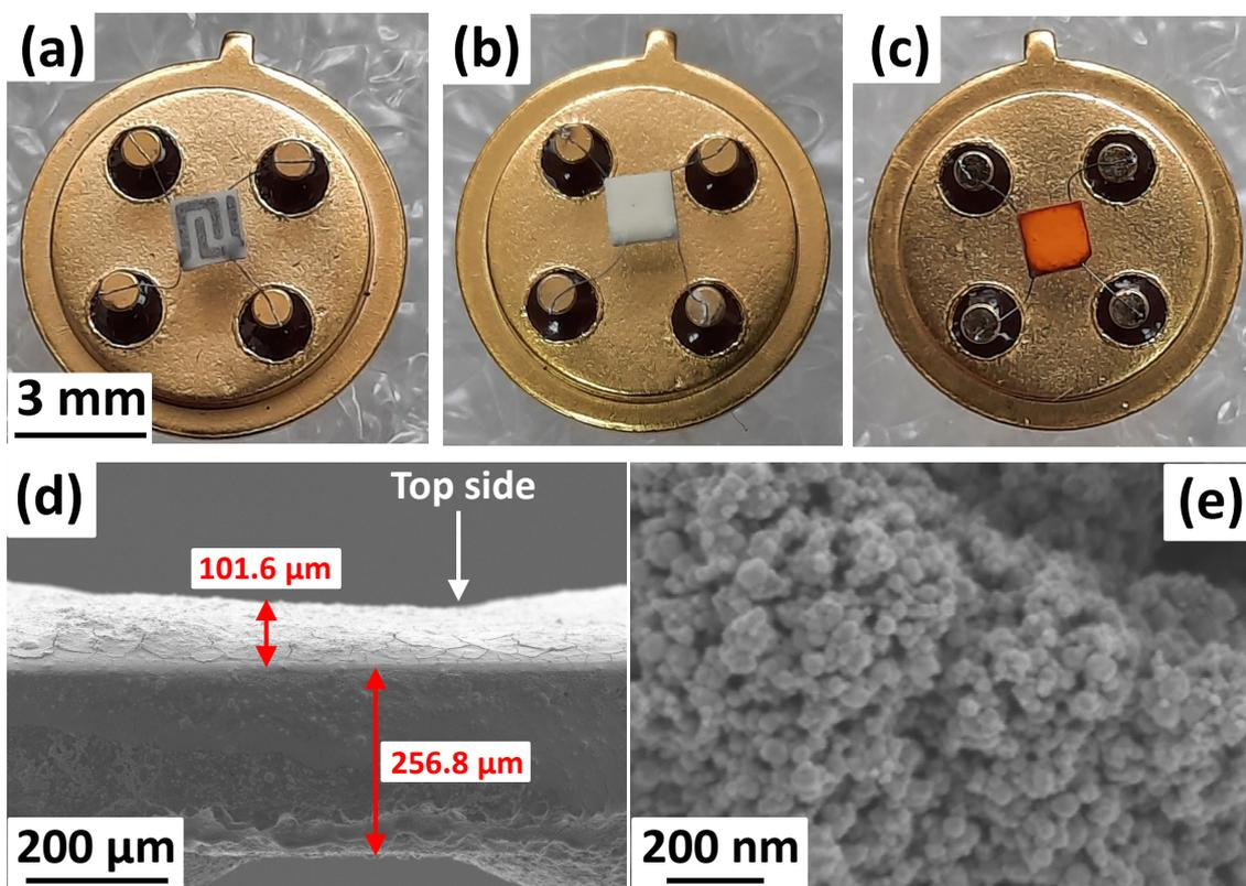
**Figure 1.** Microelectronic hotplate (a) before and (b) after deposition of a thick semiconductor film on the substrate and (c) after sensitization with a Ru(II) heteroleptic complex; SEM images of the sensitive layer deposited on the substrate, (d) side view and (e) top view.
