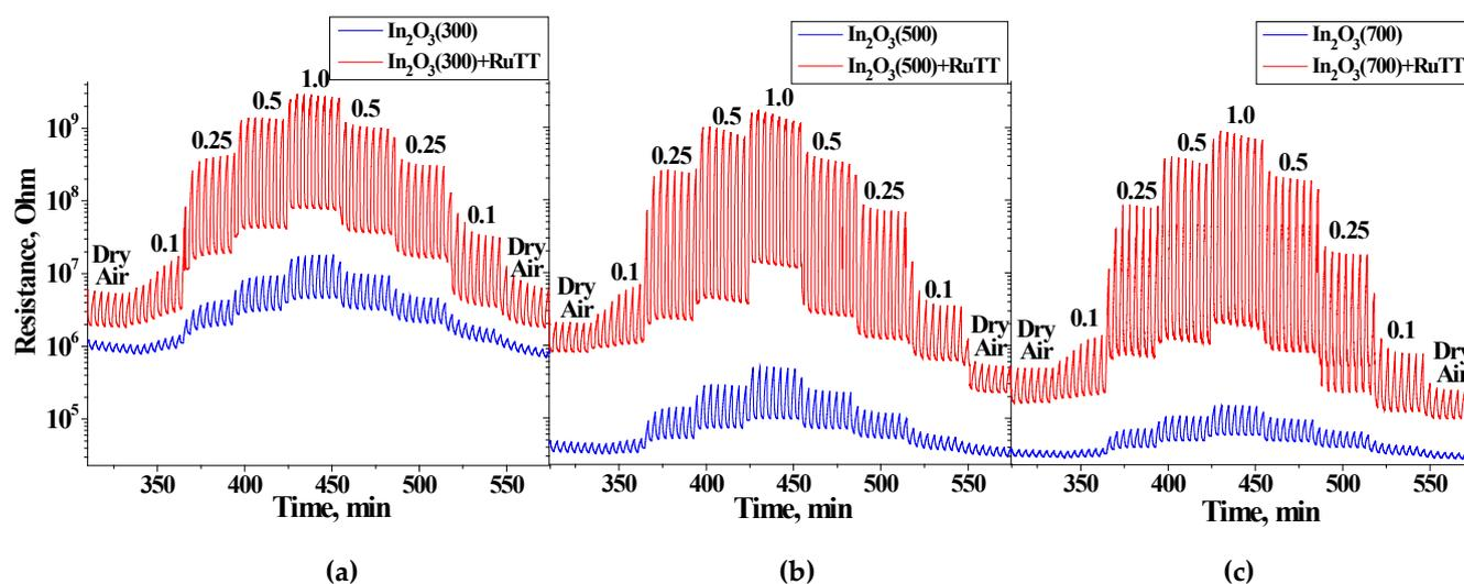
**Figure 8.** Change in resistance of the pure oxides and hybrid materials under periodic illumination with blue LED in the presence of various  $\text{NO}_2$  concentrations for (a)  $\text{In}_2\text{O}_3(300)$  based, (b)  $\text{In}_2\text{O}_3(500)$  based, (c)  $\text{In}_2\text{O}_3(700)$  based samples.
