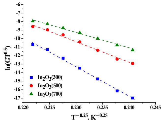
**Figure 4.** Temperature dependence of conductivity of the In<sub>2</sub>O<sub>3</sub>(300), In<sub>2</sub>O<sub>3</sub>(500) and In<sub>2</sub>O<sub>3</sub>(700) samples in Mott coordinates in the temperature range of 140–25 °C.
