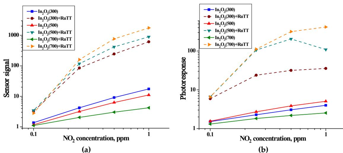
**Figure 9.** Dependence of the sensor signal (a) and photoresponse (b) of  $\text{In}_2\text{O}_3(300)$ ,  $\text{In}_2\text{O}_3(500)$ ,  $\text{In}_2\text{O}_3(700)$  samples and hybrid materials based on them on the concentration of  $\text{NO}_2$ .
