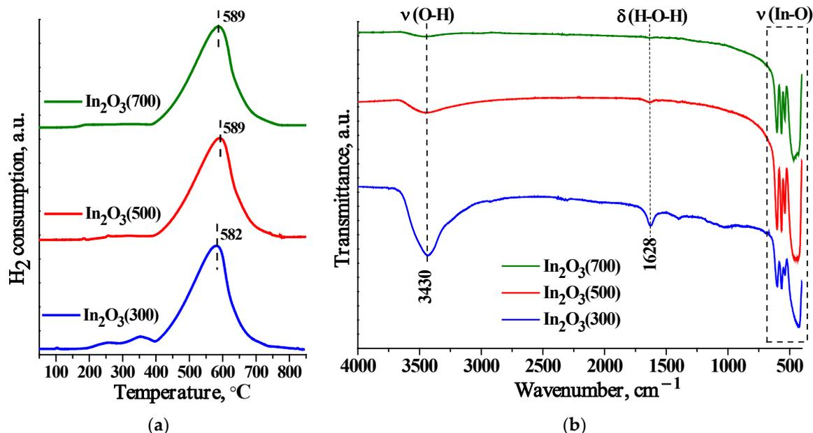
**Figure 3.** TPR-H<sub>2</sub> curves (a) and FTIR spectra (b) of nanocrystalline In<sub>2</sub>O<sub>3</sub> samples with different annealing temperatures.
