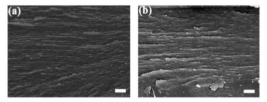
**Figure 5.** SEM images of fractured surface of (**a**) CLC film and (**b**) CLC-PAA photonic crystal hydrogel film when the films were cut perpendicularly to the surface of films. scale bar:  $1 \mu m$ .
