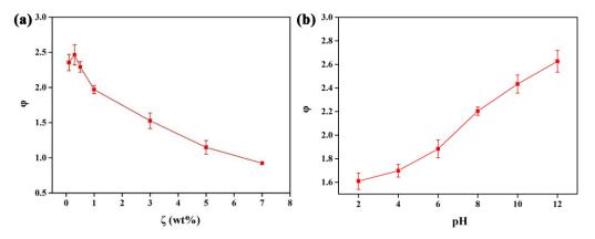
**Figure 3.** Swelling ratio ( $\phi$ ) of PAA gel film (**a**) at different amounts of TPGDA ( $\zeta$ ) and (**b**) at different pH.  $\phi$  is defined as  $(m_2 - m_1)/m_1$ , where  $m_2$  and  $m_1$  are the mass of gel film in water and dry state, respectively.
