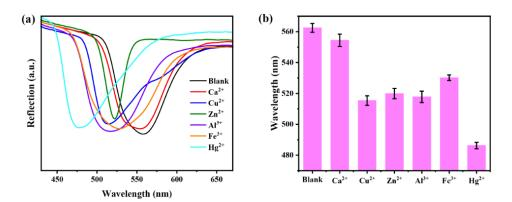
**Figure 12.** (a) UV-visible reflection spectra of CLC-PAA<sub>urease</sub> PC films with various metal ions (The films were treated with urea (10 mM) for 10 min); (b) The wavelength values of the reflected light of CLC-PAA<sub>urease</sub> PC films with various metal ions.
