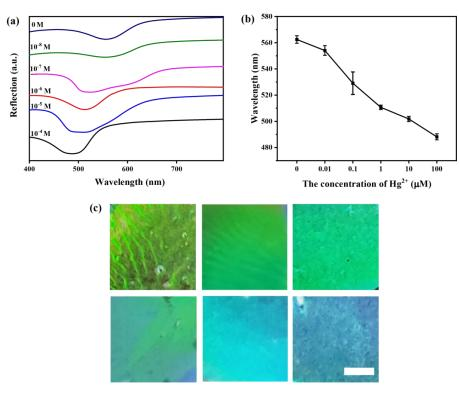
**Figure 11.** (a) The UV-visible reflection spectra of CLC-PAA<sub>urease</sub> PC films at different concentrations of  $Hg^{2+}$  (The films were treated with 10 mM urea for 10 min.); (b) The wavelength values of the reflection light of CLC-PAA<sub>urease</sub> PC films at different concentrations of  $Hg^{2+}$ ; (c) The optical images of CLC-PAA<sub>urease</sub> PC films at different concentrations of  $Hg^{2+}$ . scale bar: 1 mm.
