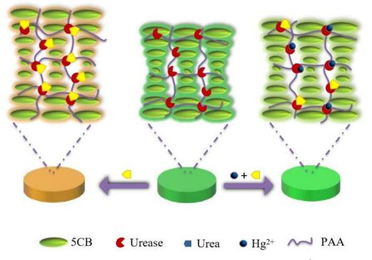
Figure 1. Schematic diagram of CLC-PAA urease PC films for the detection of Hg<sup>2+</sup>.
