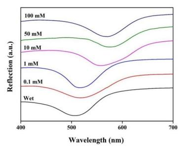
**Figure 9.** UV-visible reflection spectra of CLC-PAA<sub>urease</sub> photonic crystal hydrogel films after dropping urea solution (200  $\mu$ L) with different concentrations for 10 min.
