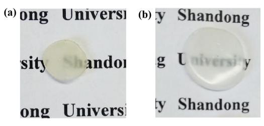
Figure 2. Comparison diagram of PAA gel film in water: (a) before and (b) after the swelling.
