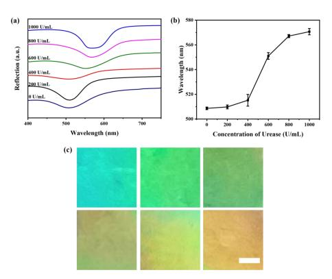
**Figure 10.** (a) The UV-visible reflection spectra of CLC-PAA PC films at different concentrations of urease (The films were treated with 10 mM urea for 10 min.); (b) The wavelength values of the reflection light; (c) The optical images of CLC-PAA PC films at different concentrations of urease. scale bar: 1 mm.
