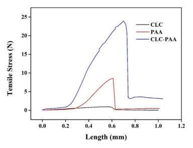
Figure 6. Tensile stress-strain curves of CLC, PAA and CLC-PAA films.
