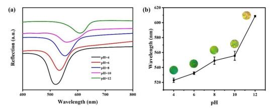
**Figure 7.** (**a**) UV-visible reflection spectra of CLC-PAA PC films at different pH; (**b**) The wavelengths of the reflection light and the optical images of CLC-PAA PC films under different pH.
