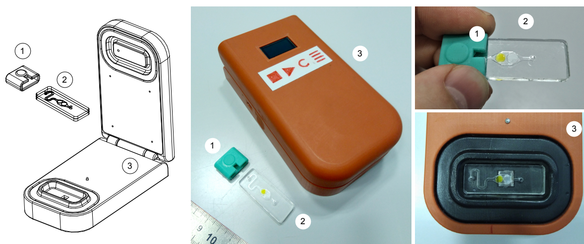
Figure 1. The biosensor consists of a SiPM-based handheld luminometer (3), a disposable microfluidic chip (2) and a sampler adapter for chips (1). The portable luminometer has the capability of autonomous operation, for this purpose it is equipped with a battery, a display and control buttons. The disposable microfluidic chips contain enzymes and substrates of the coupled enzyme bioluminescent system NAD(P)H:FMN-oxidoreductase+Luciferase co-immobilized into starch gel.
