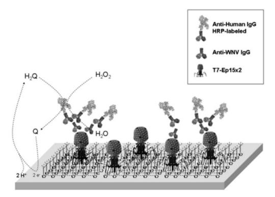
**Figure 15.** Scheme of T7 bacteriophage-based sensor for anti-WNV antibodies detection. WNV-epitope-carrying T7 phages are immobilized in the layer of conducting polymer. If the specific antibodies are present in the sample, they are bounded in a sandwich complex between a phage and a secondary antibody conjugated with an enzyme whose product is amperometrically detected [121]. Reprinted with permission from [121]. Copyright 2007 American Chemical Society.
