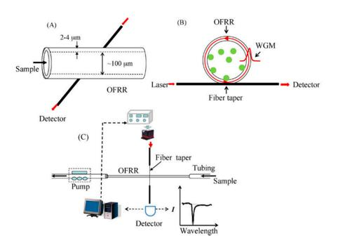
**Figure 11.** Scheme of optofluidic ring resonator (OFRR) sensor. (**A**) OFRR consists of a glass capillary with an ultra-thin wall (2–4 nm) and lumen about 100 μm in diameter. (**B**) Whispering gallery modes (WGMs) may be investigated by a laser directed on the OFRR. (**C**) Schematic of the apparatus required to run an OFRR sensor. [62] Reprinted from [62], Copyright 2008, with permission from Elsevier.
