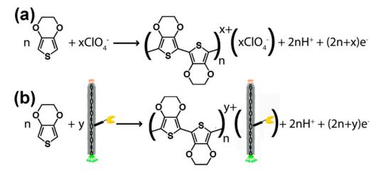
**Figure 6.** Scheme of the electropolymerization of EDOT (3,4-ethylenedioxythiophene) (**a**) in  $\text{LiClO}_4$  and (**b**) in phage solution. Both negatively charged individuals are embedded in the polymer structure. The yellow 'pacman' symbolizes PSMA-binding peptide exposed on the pVIII major coat protein of phage. Reprinted with permission from [82]. Copyright 2012 American Chemical Society.
