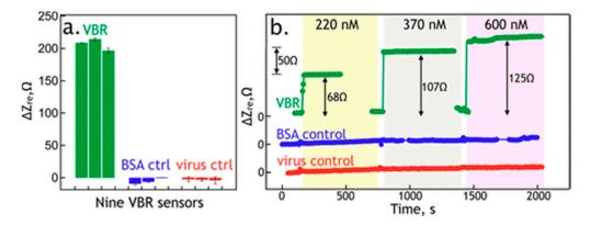
**Figure 8.** (a) Selectivity of the human serum albumin (HSA) virus bioresistor sensors against bovine serum albumin (BSA) (VBR sensor operated in a solution of BSA instead of HSA) and the control (PEDOT layer containing wild type phages do not bind HSA), (b) VBR sensor response (real impedance change) for varied HSA concentrations, control BSA probes and wild-type virus were applied as in (a). Reprinted with permission from [60]. Copyright 2018 American Chemical Society.
