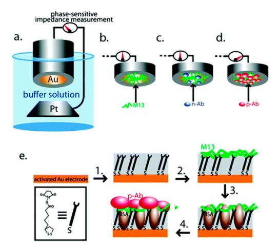
**Figure 3.** Scheme of a virus-based electrochemical sensor. Scheme of the measuring system (**a**) and reference state of the M13 virus-based electrode (**b**). The surface of a gold electrode is functionalized according to (**e**) 1–3. Sensor response (measured via EIS) is specified to the target—positive antibody, p-Ab (**d**)—and is negligible for a non-specific target—negative antibody, n-Ab (**c**). Reprinted with permission from [55]. Copyright 2006 American Chemical Society.
