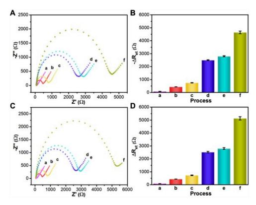
**Figure 4.** Impedimetric prostate-specific membrane antigen (PSMA) sensor fabrication (a–e) and operation (f): Nyquist plots (**A**), (**C**) and corresponding charge transfer resistance calculated using the alternative circuit. (**A**,**B**) correspond to one specific phage clone, whereas (**C**,**D**) present result for another phage clone applied in the sensor. Reprinted from [58], Copyright 2019, with permission from Elsevier.
