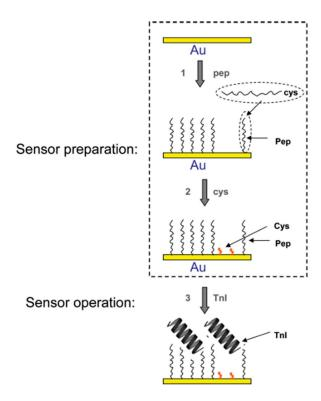
**Figure 5.** Scheme of peptide-based electrochemical sensor construction basing on a troponin I (TnI) sensor. Subsequent stages include: (1) the immobilization of cysteine-labeled affinity peptides and (2) blocking with cysteine. Operation of the sensor consists of incubation with the target's solution (3) and electrochemical measurement in the electroactive depolarizer solution. Reprinted with permission from [65]. Copyright 2010 American Chemical Society.
