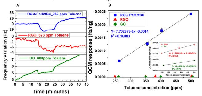
**Figure 5.** QCM sensor response of the GO, RGO, and RGO/PcH<sub>2</sub>tBu exposed to toluene (**A**); calibration curves corresponding to exposure sequences in the 250–500 ppm range (**B**).
