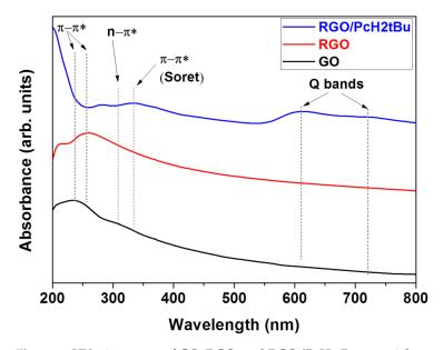
Figure 1. UV-vis spectra of GO, RGO, and RGO/PcH<sub>2</sub>tBu materials.
