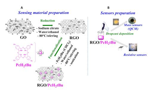
Scheme 1. Chart showing the protocol used for the material (A) and sensor preparation (B).
