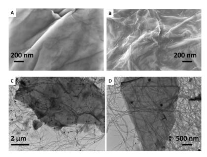
**Figure 3.** SEM images of RGO (**A**) and RGO/PcH<sub>2</sub>tBu (**B**) and TEM images of RGO/PcH<sub>2</sub>tBu at lower (**C**) and higher (**D**) levels of magnification.
