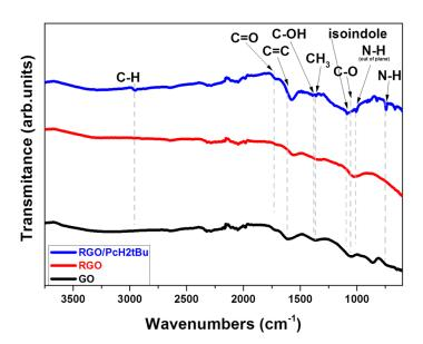
Figure 2. FTIR spectra of the GO, RGO, and RGO/PcH<sub>2</sub>tBu materials.
