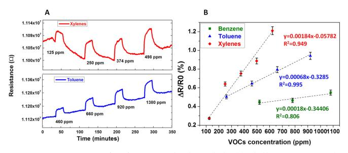
**Figure 8.** Resistive sensor response of RGO/PcH<sub>2</sub>tBu exposed to toluene and xylene (**A**) and calibration curves corresponding to the resistive sensor response of RGO/PcH<sub>2</sub>tBu exposed to benzene, toluene, and xylene (**B**). In the case of benzene, no stable and exploitable response could be obtained under 500 ppm.
