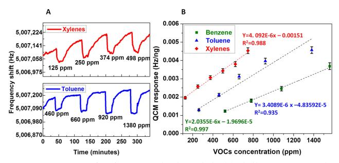
**Figure 6.** QCM sensor response of RGO/PcH<sub>2</sub>tBu exposed to toluene and xylene (**A**) and calibration curves corresponding to the QCM sensor response of RGO/PcH<sub>2</sub>tBu exposed to benzene, toluene, and xylene (**B**).
