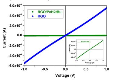
**Figure 4.** Current-voltage characteristic curves for RGO and RGO/PcH<sub>2</sub>tBu. The inset shows a magnification of the RGO/PcH<sub>2</sub>tBu, showing a higher resistance value.
