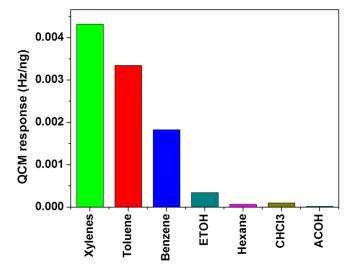
**Figure 7.** Cross-sensitivity result for the RGO/PcH<sub>2</sub>tBu exposed to BTX and to other VOCs at 750 ppm.
