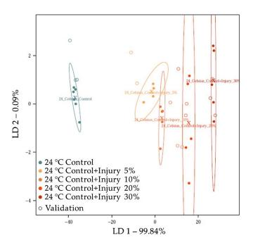
**Figure 6.** LDA classification models on the e-tongue data of raw plum juice mixtures with second parallel sample validation when the "24 °C Injury" fruit content was used as class variable (N = 39).
