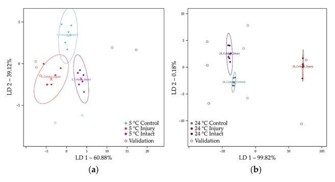
**Figure 5.** LDA classification model on the e-tongue data of control and infected plum juices with external validation when the inoculation mode was used as class variable: (**a**) LDA of samples stored at 5 °C (N = 25); and (**b**) LDA of samples stored at 24 °C (N = 26).
