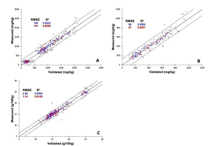
**Figure 3.** Performance of partial least square (PLS) model using the spectral data pre-treated by SNV. Calibration and external validation for total flavonoids using 9 factors (**A**), for Total Anthocyanins using 3 factors (**B**), and for Total Soluble Solids using 10 factors (**C**). Blue dots indicate calibration set and red dots represent validation set. R<sup>2</sup>: determination coefficient, RMSE: root mean squared error.
