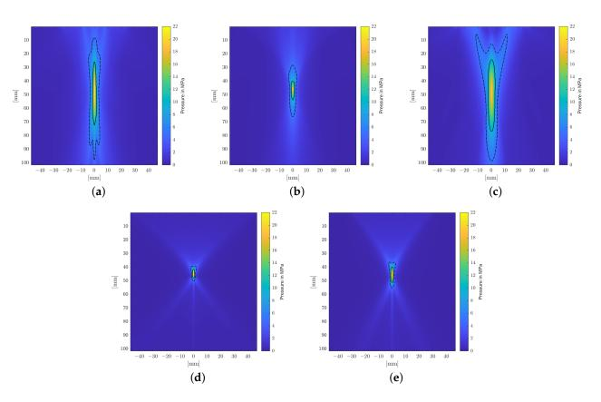
**Figure 5.** Longitudinal cross-section of the sound field showing peak pressure in a reference water bath. The -6 dB and 5 MPa focal zones are delineated by solid and dashed lines. (**a**) EH, parabolic. (**b**) EH, elliptical. (**c**) EM. (**d**) PE,  $F_{\#} = 0.68$ . (**e**) PE,  $F_{\#} = 0.87$ .
