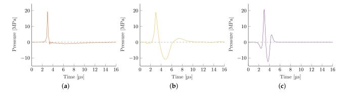
**Figure 4.** Representative simulated pressure-time curves in the water bath at the respective acoustic focus. Changes in reflector geometry for the same generating technology yield no visually discernible differences. (a) Electrohydraulic (elliptical). (b) Electromagnetic. (c) Piezoelectric ( $F_{\#} = 0.68$ ).
