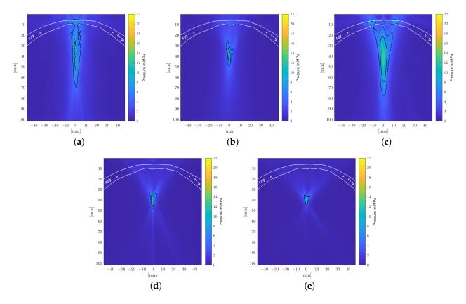
**Figure 7.** Longitudinal section of the maximal pressure in the transcranial application, using the Pichardo [41] attenuation model. The -6 dB and 5 MPa focal zones are delineated by solid and dashed lines. (a) EH, parabolic. (b) EH, elliptical. (c) EM. (d) PE,  $F_{\#} = 0.68$ . (e) PE,  $F_{\#} = 0.87$ .
