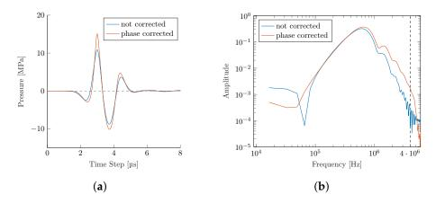
**Figure 9.** Comparison of the pressure signals and their frequency spectra for the non-corrected and phase-corrected PE transducers. (a) Signal pressure. (b) Frequency spectrum.
