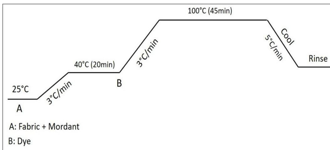
**Figure 1.** Simultaneous mordanting dyeing process.
