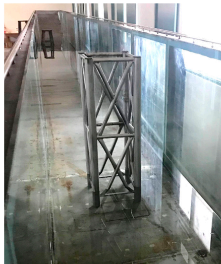
Figure 3. The scaled down testing model in the water tank for the offshore jacket-type structure.
