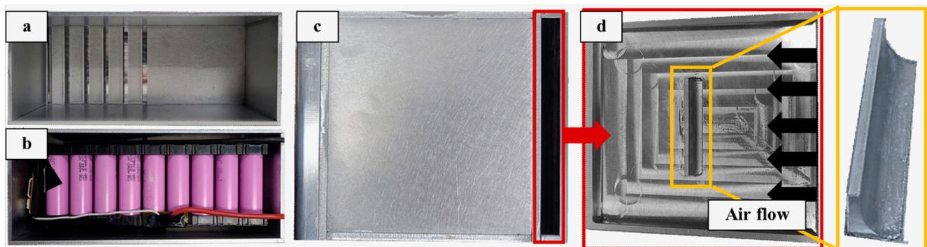
**Figure 8.** Schematics of the experimental system for the spoiler-type model: (a) inside the model; (b) schematic of assembled battery module; (c) outside the model; (d) with the spoiler at the inlet.
