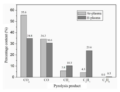
Figure 5. Columnar comparison of the pyrolysis product content of Ar-plasma and Ar/H<sub>2</sub>-plasma.
