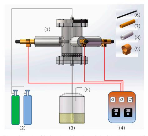
**Figure 1.** Illustration of the three-phase AC arc plasma device. (1) pyrolysis reactor; (2) gas supplier; (3) oil collector; (4) powder supplier; (5) gas collector; (6) graphite rod; (7) copper tube; (8) electrode jackets; (9) electrode connector.
