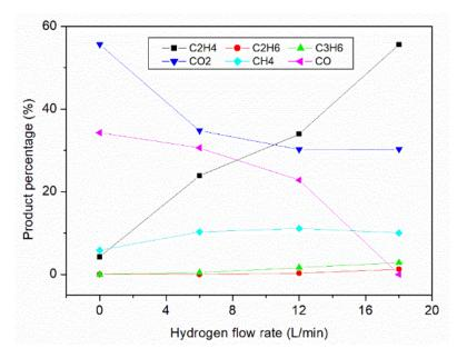
Figure 6. Effect of hydrogen flow rate on the percentage of the gas product.
