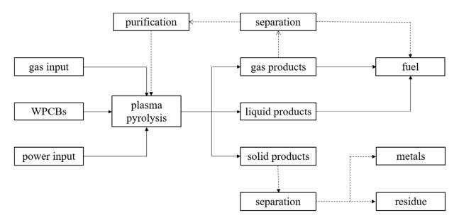
Figure 3. Scheme of the technological process in three-phase alternating arc plasma assisted utilization of WPCBs.
