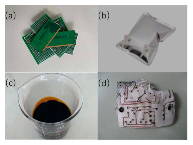
Figure 4. WPCBs (a) and the pyrolysis products in gas (b), liquid (c), and solid (d) phase.
