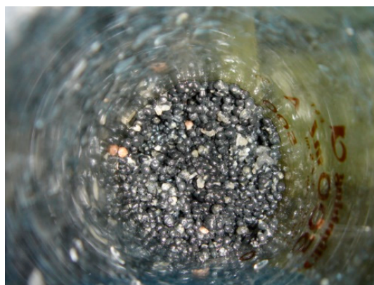
Figure 6. Granular sludge formed in the EGSB.
