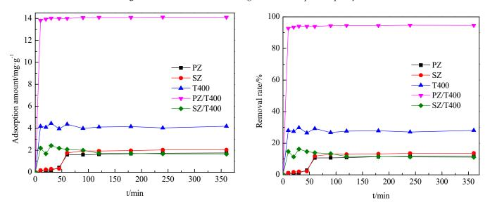
Figure 8. Effect of time on the adsorption capacity and removal rate of AB10B.
