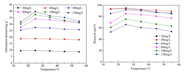
Figure 10. Effect of temperature on the adsorption capacity and removal rate of AB10B.
