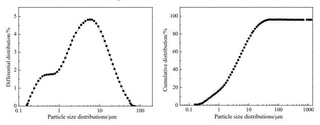
Figure 1. The particle size distribution of zinc ferrite samples before powdering.
