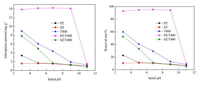
Figure 5. Effect of pH on the adsorption capacity and removal rate of AB10B.
