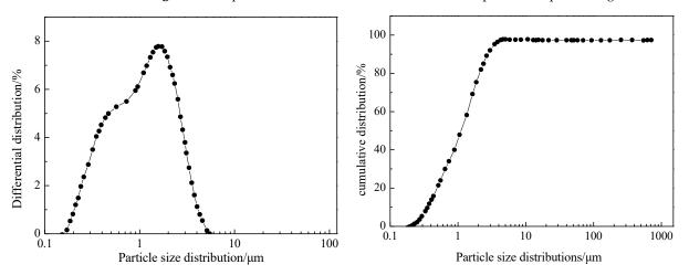
Figure 2. The particle size distribution of zinc ferrite samples after powdering.
