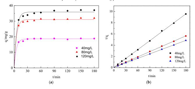
**Figure 13.** Fitting of adsorption kinetics by pseudo-first-order model (**a**) and pseudo-second-order model (**b**) for adsorption of AB10B on PZ/T400 at different initial concentrations.
