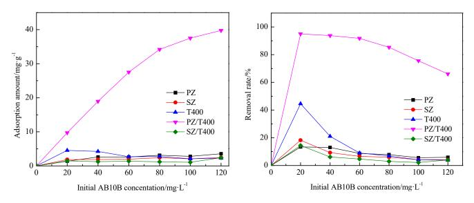
**Figure 9.** Effect of initial concentration of the solution on the adsorption capacity and removal rate of AB10B.
