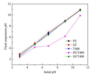
Figure 6. Changes of pH after AB10B adsorbed on various samples.
