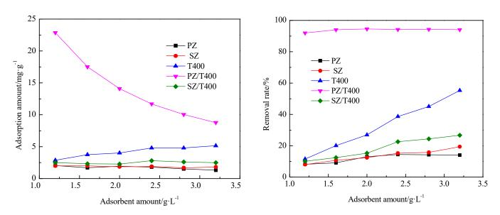
Figure 7. Effect of adsorbent dosage on the adsorption capacity and removal rate of AB10B.
