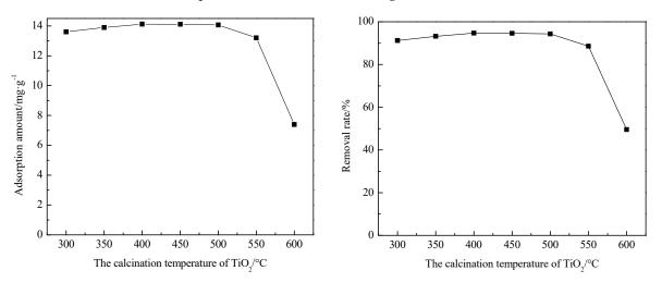
**Figure 3.** Effect of the calcination temperature of TiO<sub>2</sub> on adsorption capacity and removal rate of AB10B.
