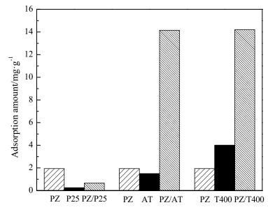
Figure 11. Effect of purified  $ZnFe_2O_4$  mixed with different  $TiO_2$  on the adsorption capacity of AB10B.
