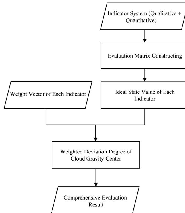
**Figure 7.** Flowchart of cloud gravity center deviation ranking method.
