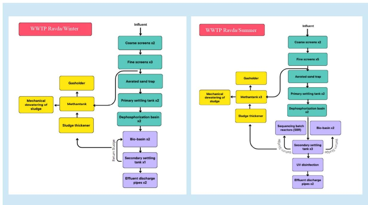
**Figure 2.** Simplified scheme of WWTP Ravda with mechanical treatment (green), biological (blue) treatment, and sludge route (yellow)—comparison between winter and summer wastewater treatment.
