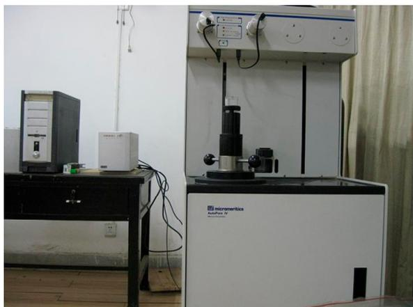
**Figure 1.** MK-AutoPore IV9510 mercury injection apparatus.
