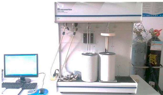
**Figure 2.** ASAP 2020M automatic analyzer for SSA (specific surface area) and micropores.
