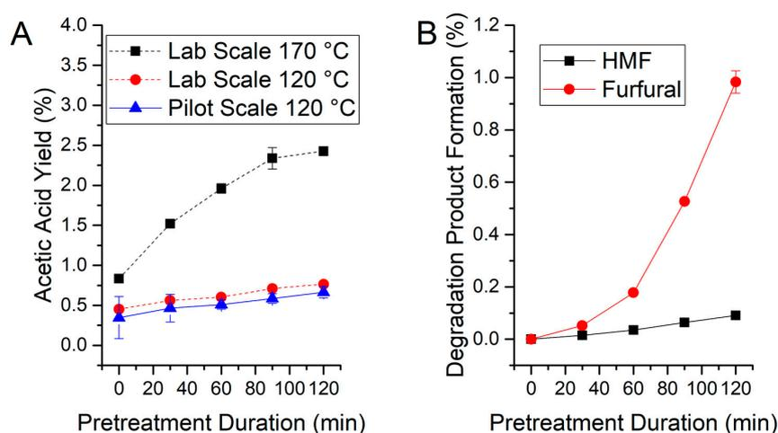
**Figure 4.** (A) Acetic acid generated during the LHW pretreatment. (B) Degradation product formation during the lab-scale pretreatments at 170 °C. Shown degradation products were below detection limit (1.3 mg/L for Furfural; 0.6 mg/L for HMF) at pretreatments at 120 °C.
