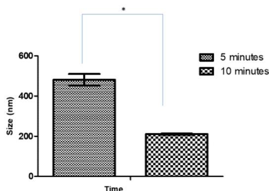
**Figure 2.** Effect of sonication time on the size of Ag-FSE CSNPs (5mg); \*significant difference with CSNP sizes ( $p < 0.05$ ).
