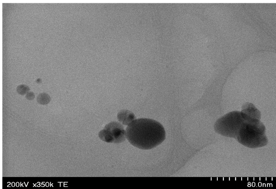
**Figure 4.** TEM images of Ag-FSE loaded CSNPs; where nanoparticles appeared globular in shape.
