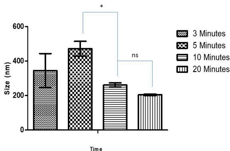
**Figure 1.** Effect of sonication time on size of blank CSNP; \* significant difference with CSNP size at 5 and 10 min sonication ( $p < 0.05$ ); ns, non-significant.
