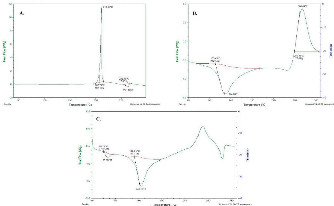
**Figure 6.** DSC results of (a) Ag-FSE, (b) CS and (c) Ag-FSE CSNPs.
